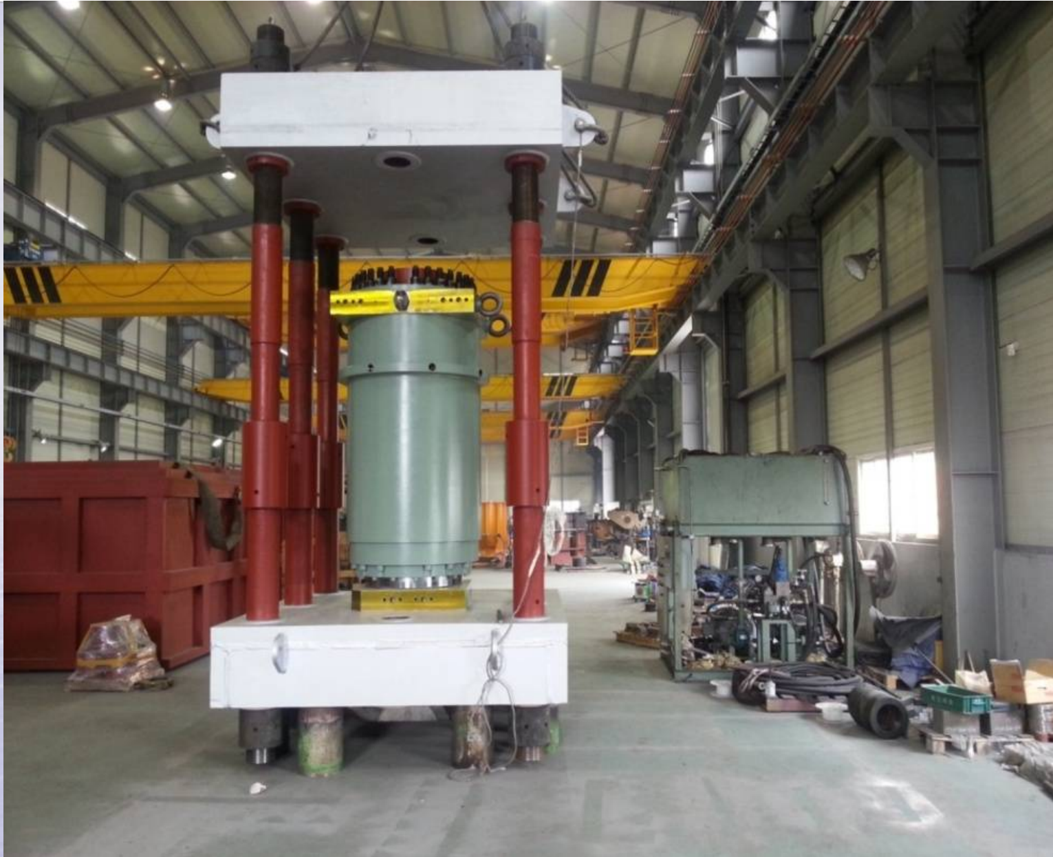
▷ LADDLE LIFTING CYL. JIG TEST (POSCO)
