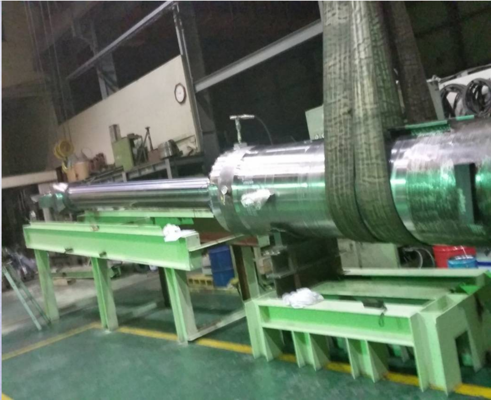
▷ CSU BOOM HOISTING CYL. SCALE 1:5 TEST (THERMOELECTRIC POWER PLANT)
