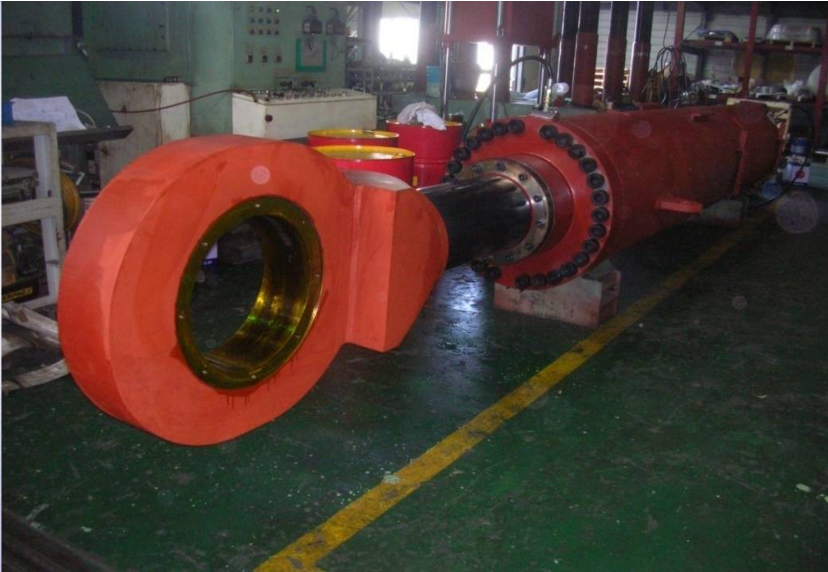
▷ CSU BOOM HOISTING CYL. MAINTENANCE (THERMOELECTRIC POWER PLANT)
